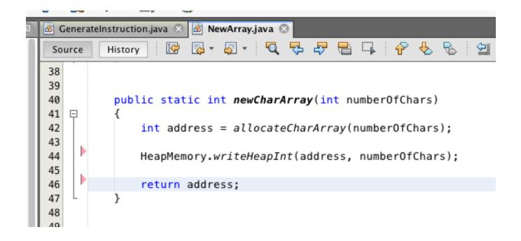
• This method runs only on the target and allocates char arrays from the heap and initializes each array with the length of the array. The presence of the length enables index range checking to verify that the bounds of the array are not being exceeded by application code.
