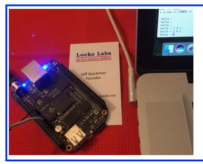
LED set command ('I 4 s') writes a 1 to the control bit, turning the LED on.
